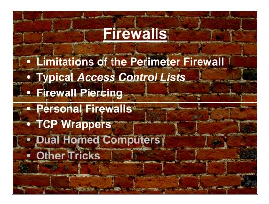
There are many different techniques to Pierce a firewall. The techniques usually involve a initiating the communication session from the inside the trusted network using a protocol that is permitted.
